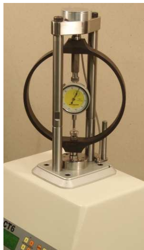
Figure 9 - Calibration Using a Proving Ring
