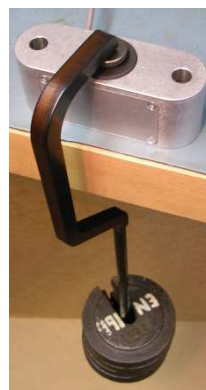
Figure 8 - Dead Weight Calibration
