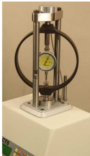
Figure 9 - Calibration Using a Proving Ring
