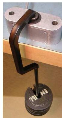
Figure 8 - Dead Weight Calibration
