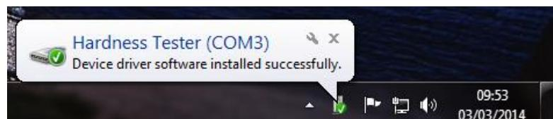
This virtual COM port will be present only when the C53 or CT6 is plugged in. If there is any doubt as to which port to use, open Device manager by right-clicking on 'Computer' and selecting 'Properties'. Click 'Device Manager' on the left-hand pane. Click the plus symbol next to 'Ports (COM & LPT)' to expand it. One of the ports listed will be 'Hardness Tester'. This will tell you which COM port to use:
